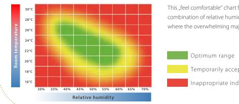
This "feel comfortable" chart for indoor room climate demonstrates the combination of relative humidity and room temperature where the overwhelming majority feels comfortable in indoor rooms.
